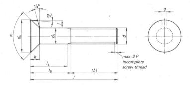
Designation of a flat countersunk nib bolt, with screw thread d=M 10, length l=70 mm and strength category 3.6 or 4.6 (at manufacturer's discretion):
