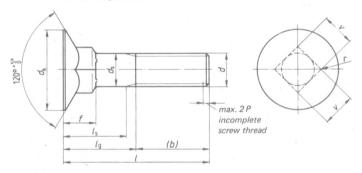
Designation of a flat countersunk square neck bolt with long square, with screw thread  $d=\mathrm{M}\ 10$ , length  $l=70\,\mathrm{mm}$  and strength category 3.6 or 4.6 (at manufacturer's descretion):
