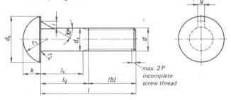
Designation of a cup head nib bolt, with screw thread  $d={\rm M}~10$ , length  $l=70~{\rm mm}$  and strength category  $3.6~{\rm or}~4.6$  (at manufacturer's discretion):
