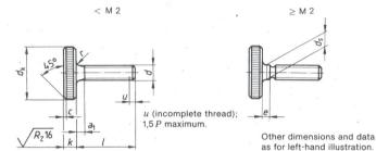
Where knurled thumb screws of sizes not less than M2 shall be supplied threaded up to the head, letter A as specified in
